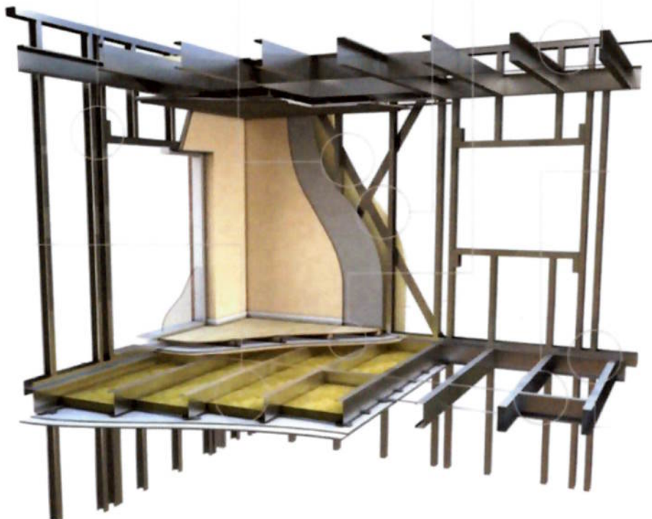
Figure 25 – Typical Metsec SFS System
